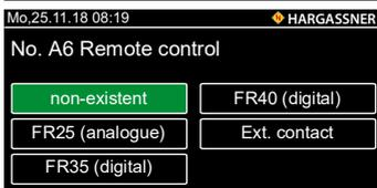
No. A6 Heat circuit 1 and 2 remote control , 5 setting options:
