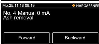
No. 4 Function and rotation check of ash extraction motor
