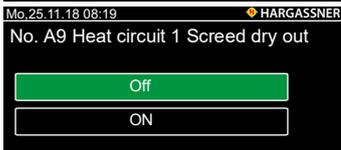
No. A9 Activation of screed heating function of the corresponding heat circuit
