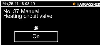
No. 37 Function and rotation check on the heat circuit valve
