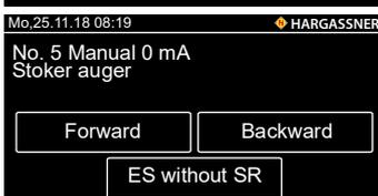
No. 5 Function and rotation check of stoker auger motor
